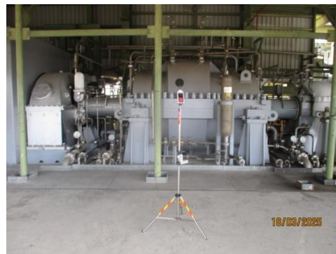
Cracked Gas Compressor (R-3301)
