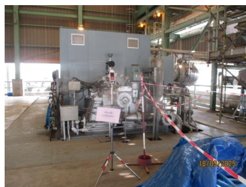
Propylene Compressor (R-650)
